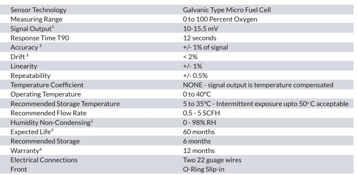
Note: SRZ-CF25F4 is without flange top and O-ring front. Do not expose sensor to temperatures above 50°C for extended period of time. Failure to do so may have negative impact on its performance and life.
