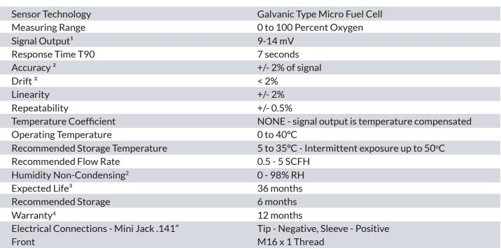
**Note:** SRX-CT-2 is designed as a component for breathing air equipment, user must verify its compatibility with intended equipment. For optimal accuracy, sensor must be calibrated before each use and after 24 hours of continuous use in oxygen above 90%. Do not expose sensor above 50°C for extended period of time. Failure to do so may have negative impact on its performance and life.
